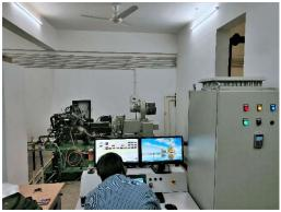
Make: Accurate Test Equipment's and Engineers Test Setup: Internal combustion engine with transient dynamometer
