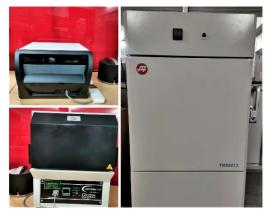
Make: Hot Disk Model: TPS 2500S Applications: To measure Thermal conductivity of material Specifications:
