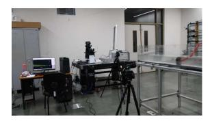
Make: Microvec Model: PIVotal-200 Applications: Used to measure fluid flow patterns and velocities. Specifications:
