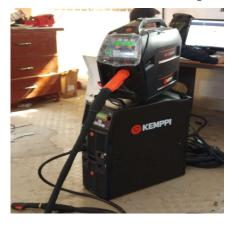
Make: Kemppi India Private Limited Model: Fast MIG X450c Applications: Welding thin/thick materials, Additional features such as root wise, root thin, scratch TIG etc.
