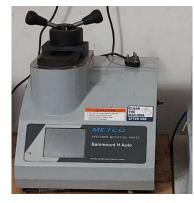
Make: Chennai metco Model: MPH007A Applications: Fully automatic hydraulic hot mounting press for various characterisation Specifications:
