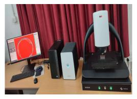
Make: INNOVATEST Model: FALCON 502 Applications: Hardness measurement. Specifications:
