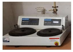
Make: Chennai metco Model: PMV018 Applications: Grinding and Polishing of materials for metallurgical application Specifications:
