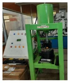
Make: ETA Technology Pvt. Ltd. Model: ETA /WS007 Applications: Friction stir welding, processing and solid-state additive manufacturing Specifications:
