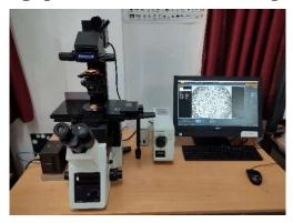
Make: Olympus medical system India Model: Olympus IX 73 Applications: Used for high-resolution live cell imaging and observation. Specifications:
