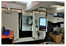
Make: DMG MORI Asia Pvt. Ltd. Model: DMG MORI/CLX350 V3 Applications: Turning, Thread cutting, Grooving, Drilling, Indexing, Boring, Chamfering and end milling. Specifications:
